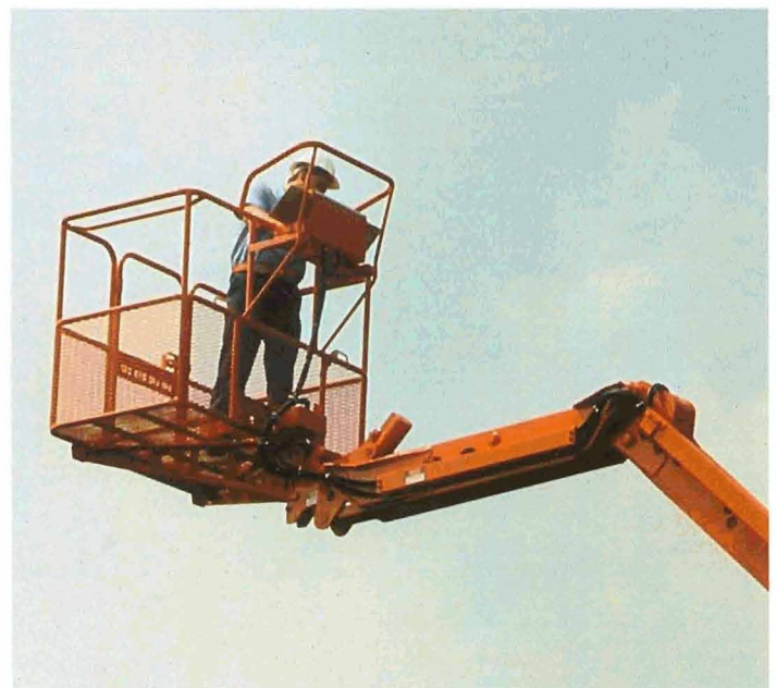
The Extend-A-Reach option articulates 15° above or 80° below horizontal of main boom to give operator "up and over" or "out and down" access.
