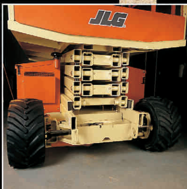
Strengthened Arm Stack for Improved Stack Rigidity
