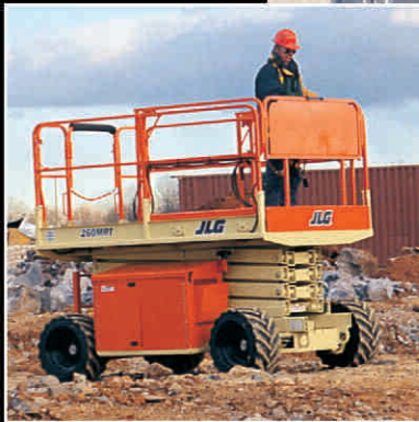
Standard Four-Wheel Drive for Terrainability
