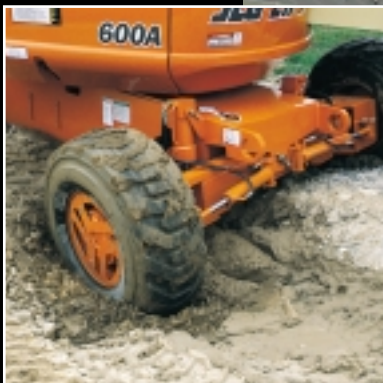
Oscillating Axle for Tough Terrain
